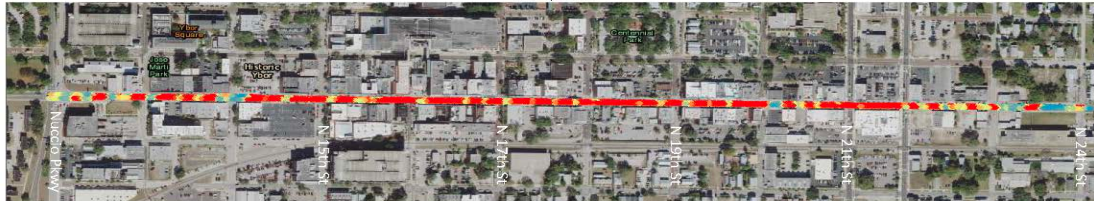
Street Lighting Level Measurement (foot candle) on 7th Avenue E
