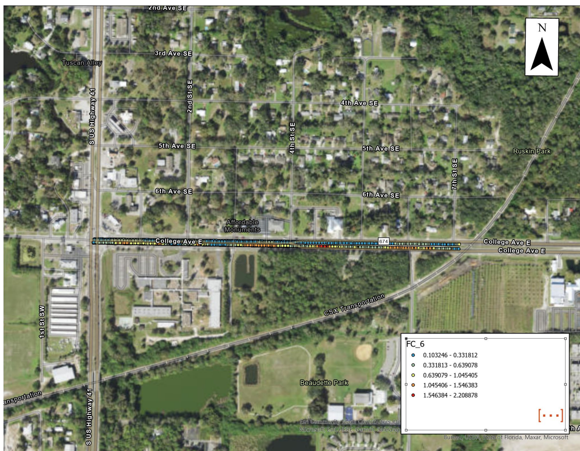
Figure 4-6. Lighting data for 0.5-mile segment
