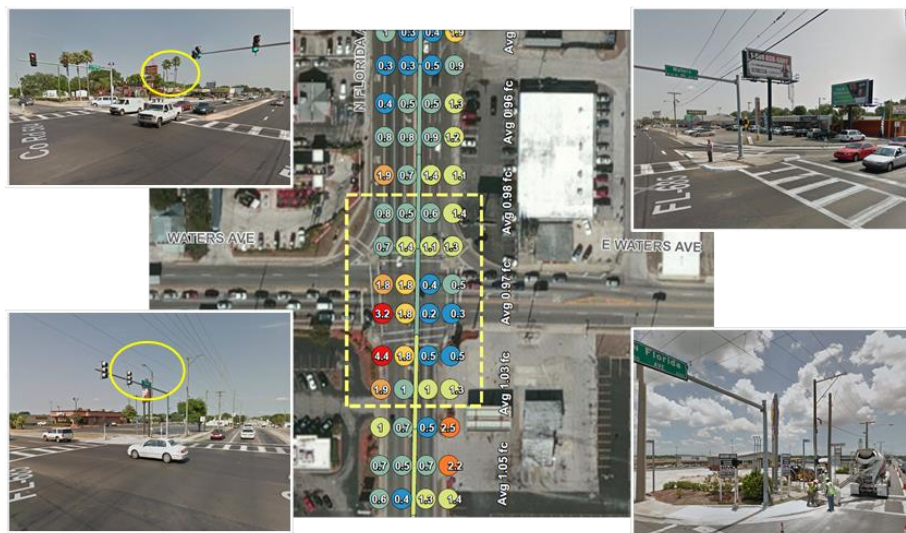
Figure 3. Examples of Horizontal Illuminance Data Collected by ALMS
